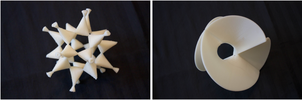
Figure 11: Photographs of 3D prints of Bertini_real decompositions. Left: Solitude. Right: the Barth Sextic. Both from a U-Print using dissolvable support material.
